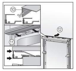
If there is a fairly large gap above the appliance, cut a wooden beam to fit exactly and place it in the gap.
